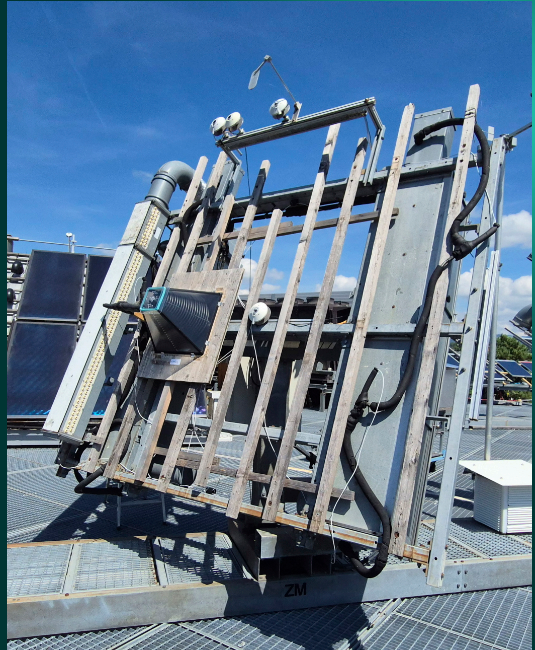
SolarisKit HelioFlow™ solar collector being tested to EN12975/ISO 9806 standards by accredited solar test lab in Switzerland.
